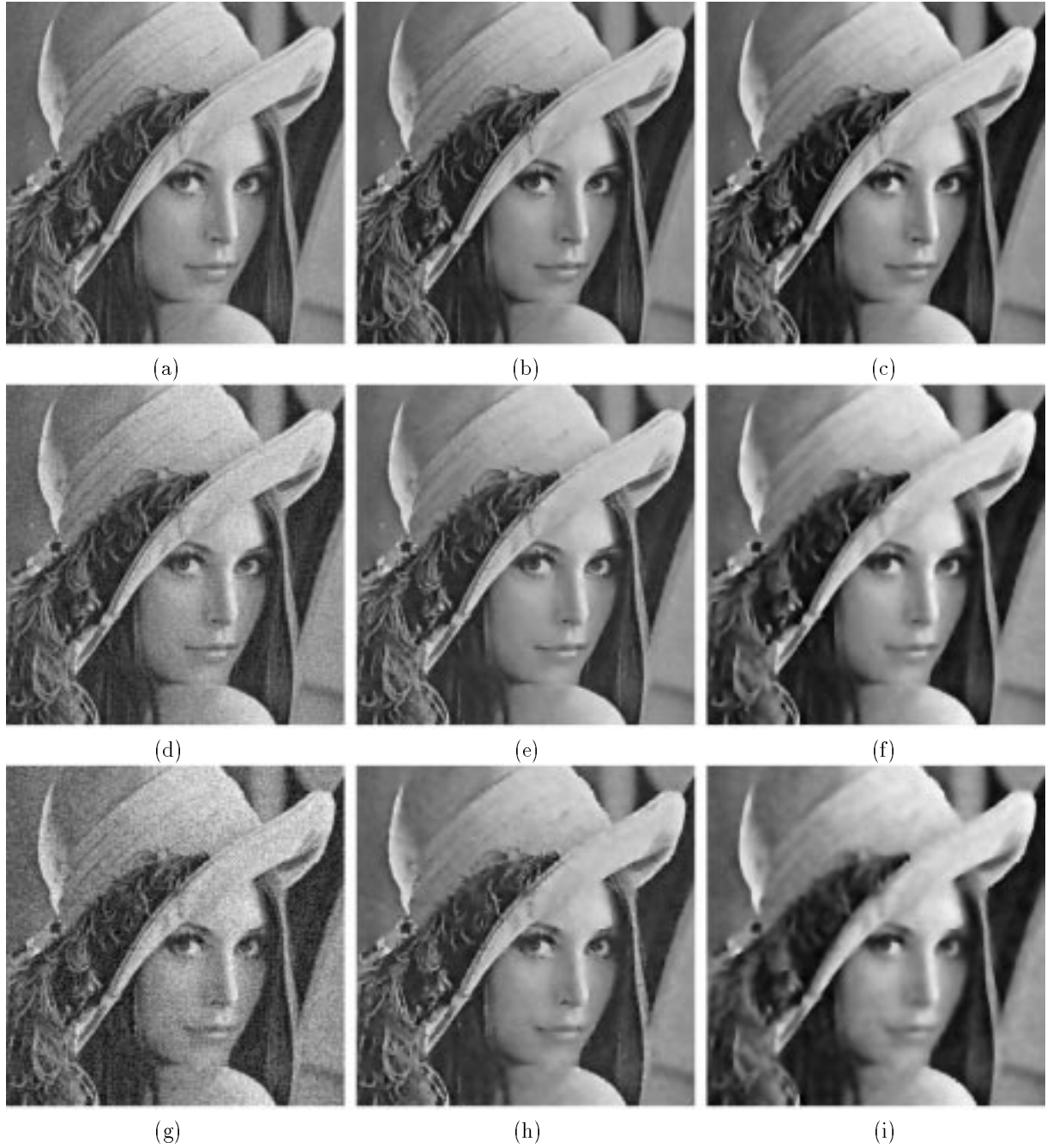
Figure 3. Comparison between Catte's operator and the new operator. The mechanism of noise addition is pixelwise adding a random number which is uniformly distributed on some interval [-\beta, \beta] . (a) Lena with uniform noise on [-15, 15] . (b) a filtered by the new operator, T = 1.6 . (c) a filtered by Catte's operator. (d) Lena with uniform noise on [-30, 30] . (e) d filtered by the new operator, T = 3.4 . (f) d filtered by Catte's operator. (g) Lena with uniform noise on [-50, 50] . (h) g filtered by the new operator, T = 4.6 . (i) g filtered by Catte's operator.
