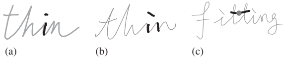
Fig. 16. Examples of dots and bars and their stem candidates. (a) A dot has only one stem candidate. (b) A dot has two stem candidates. (c) A bar has two stem candidates. It should be divided into two sub-bars in order to be bound with the two stems.
