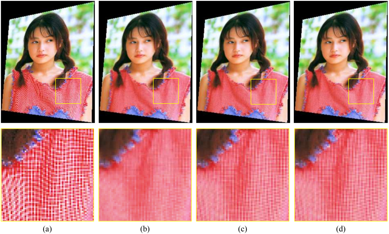
Figure 6. Texture filtering on a perspective plane with a real picture. (a) Using cubic kernel. (b) Using the EWA filter. (c) Using our NEI filter. (d) Using our FOA filter.
