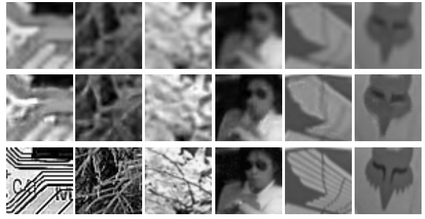
Figure 4. Part of the SR results using Sun et al.’s algorithm [15]. The magnification factor is 3.0. On the top are the LRIs of 16 \times 16 , interpolated to 48 \times 48 using bicubic interpolation. In the middle are the SR results. At the bottom are the ground truth HRIs.
