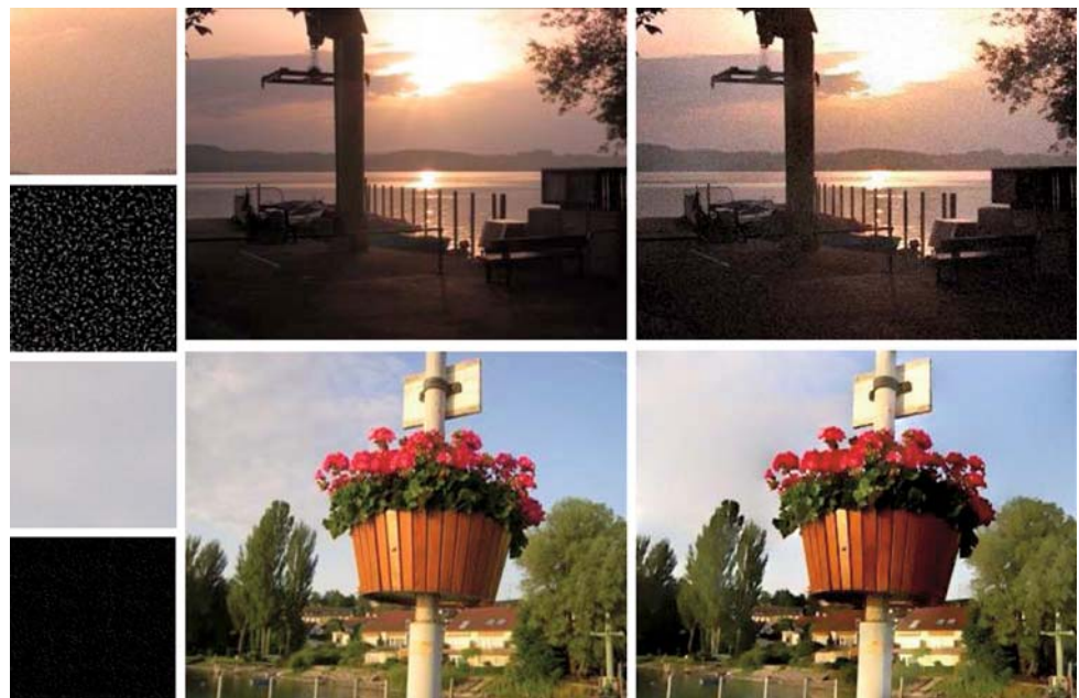
Fig. 9 Examples of image noise visualization. The first row shows the results for an original noisy image. The upper blowup is one uniform region in the noisy image, while the lower blowup shows the detected noise map in this region. The central image is the result after naïve image reduction. The right image adds the noise to the structure enhanced image according to the detected noise map. The second row shows the results for an originally clean image. The result after noise visualization still looks clean as expected
