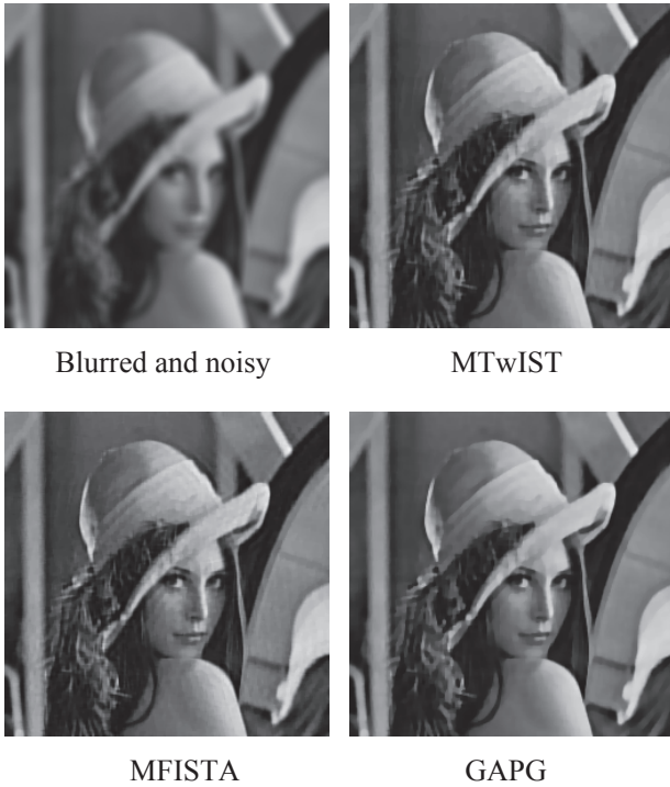
Fig. 1. Isotropic TV-based image restoration from a blurred and noisy Lena image. top left: blurred and noisy Lena; top right: restored image using MTwIST; bottom left: restored image using MFISTA; bottom right: restored image using GAPG.
