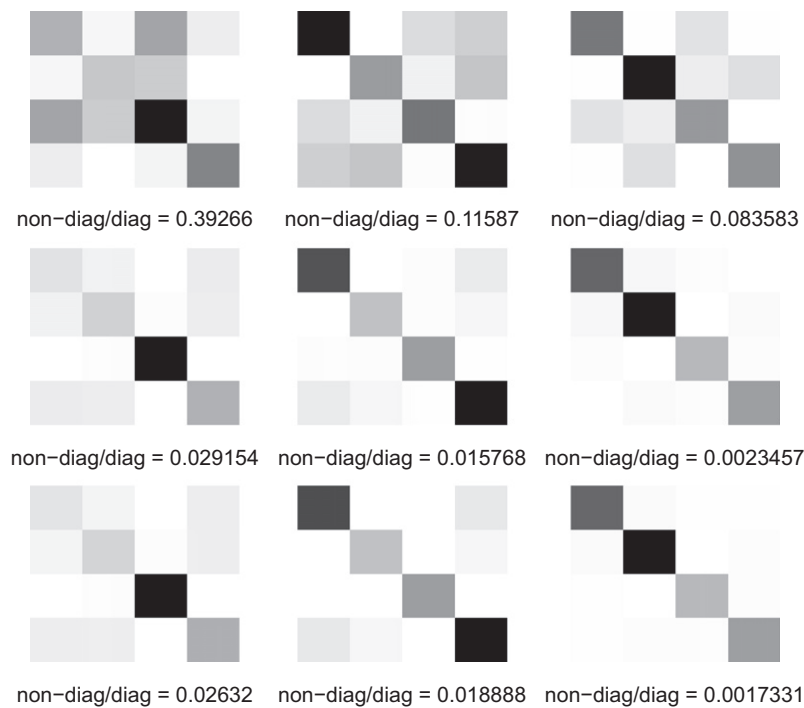
Fig. 2. Comparison of the effectiveness of simultaneously diagonalizing the class covariance matrices of two JD algorithms: the first row shows the three class covariance matrices of the IRIS data samples, the second row shows the corresponding class covariance matrices after performing Ziehe et al.'s JD algorithm, and the third row shows the corresponding class covariance matrices after performing our JD algorithm. Below each covariance matrix is the ratio of the sum of squared non-diagonal entries to that of the diagonal ones.
