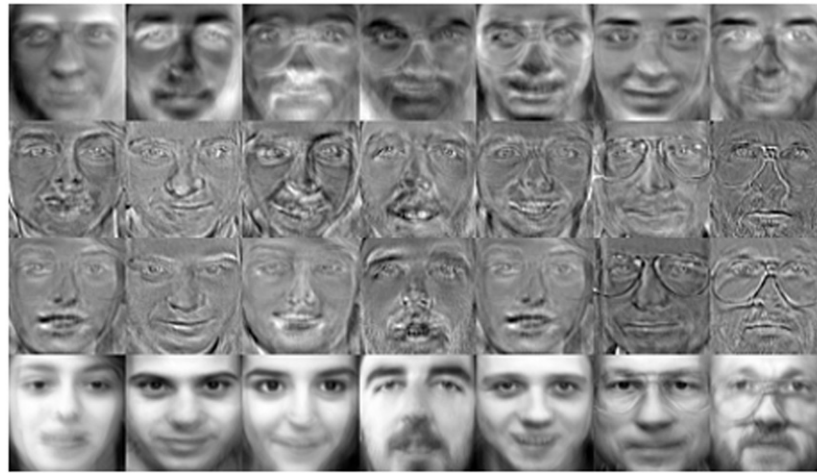
Fig. 4. Plot of the representative vectors obtained by PCA, FKT and DSA. The images in the first, second, and third rows denote the representative vectors of PCA, FKT [1], and DSA, respectively. The fourth row shows the average image of each class.
