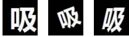
Figure 5. Examples of skewed or rotated characters. From left to right: the original image, the rotated image with a rotation angle \theta = 20 , the skewed image with a skew value t = 0.3 .
