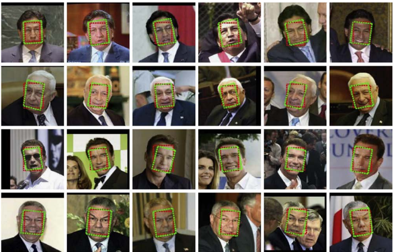
Fig. 6. Visual impression about the alignment performance of our algorithm (better viewed in color). The red bounding box indicates face images detected by the OpenCV Viola-Jones face detector. The green bounding box indicates face images aligned by our algorithm automatically. (For interpretation of the references to color in this figure caption, the reader is referred to the web version of this paper.)
