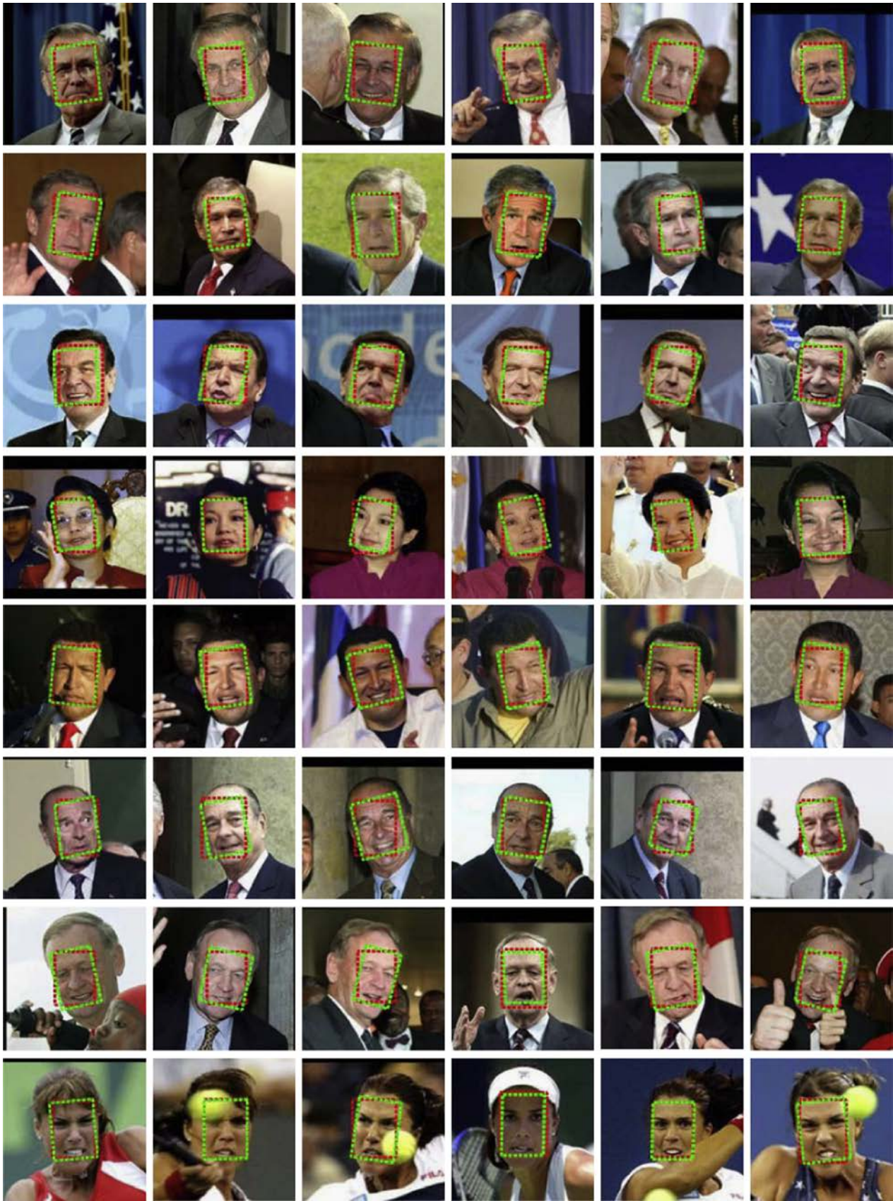
Fig. 10. More visual impression about the alignment performance on the LFW database. The red bounding box represents face images detected by the OpenCV Viola-Jones face detector. The green bounding box represents face images aligned by our algorithm automatically. (For interpretation of the references to color in this figure caption, the reader is referred to the web version of this paper.)
