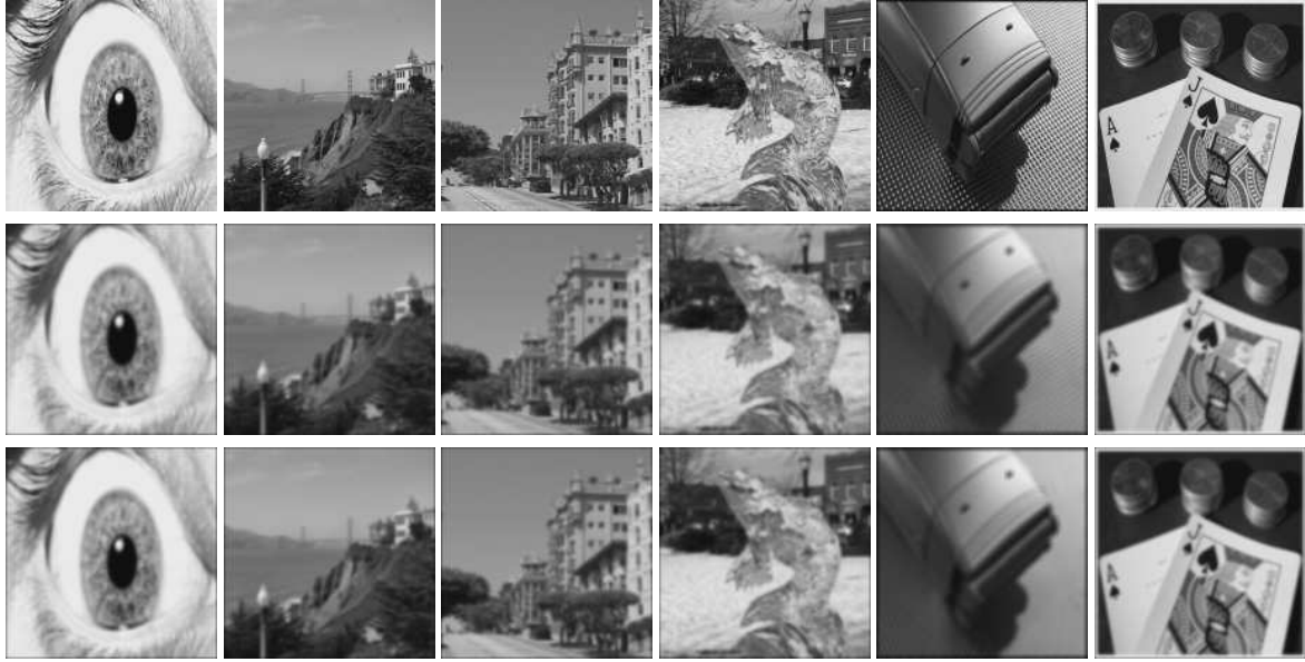
Figure 1: Partial results of image blurring. The top row are the input images. The middle row are the outputs of our learnt PDEs. The bottom row are the ground truth images obtained by blurring the input image with a Gaussian kernel. One can see that the output of our PDEs is visually indistinguishable from the ground truth.
