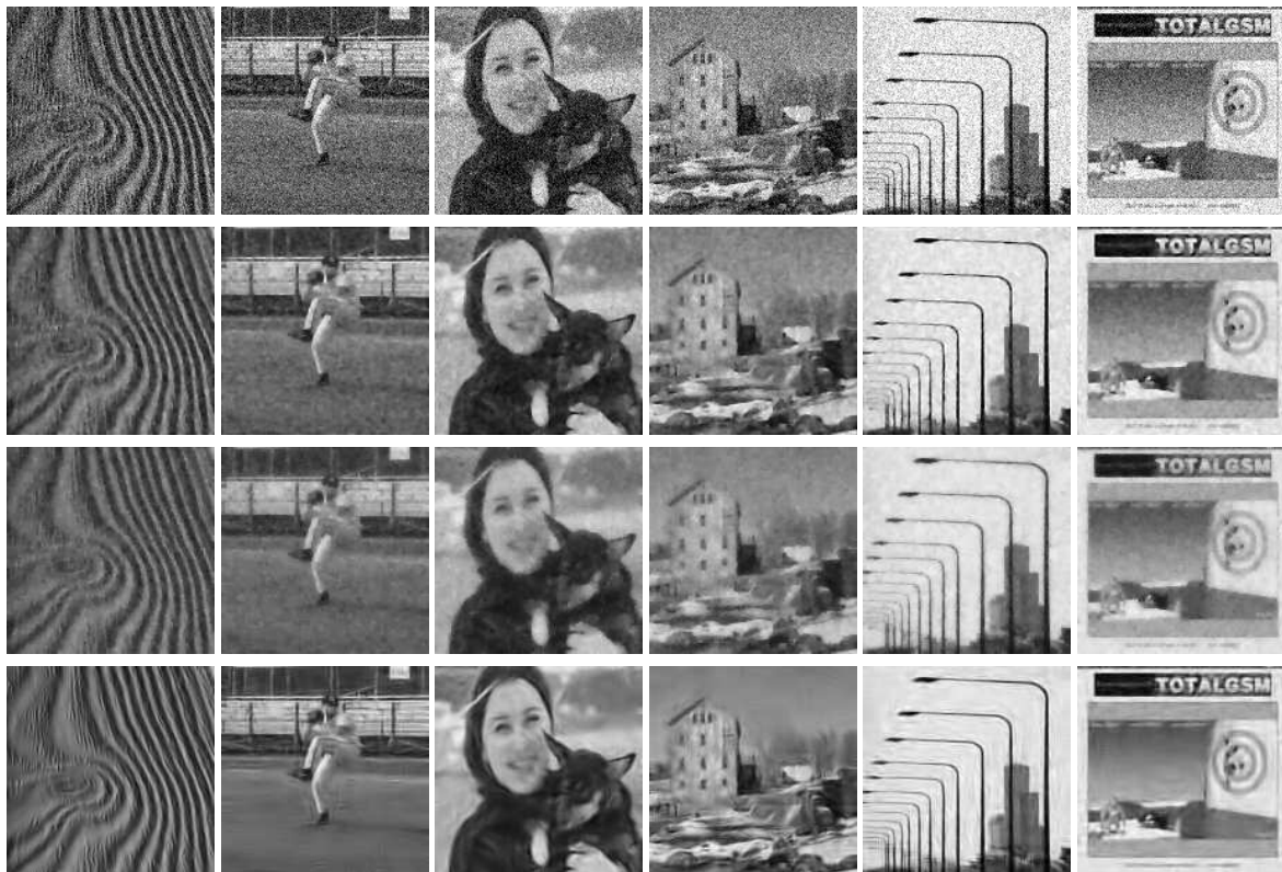
Figure 5: Partial results of image denoising. The top row are the input noisy images. The second row are the outputs of our learnt PDEs. The third row are the outputs by the ramp preserving complex diffusion method [10] (using the original code by the authors, with parameters being tuned such that the average PSNR is the highest). The fourth row are the outputs of the BLS-GSM method [24] (using the original code by the authors).
